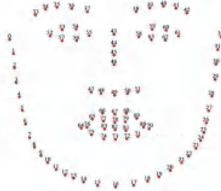
Figure 2: Face key points data detected by the ASM labeled by number sequence
